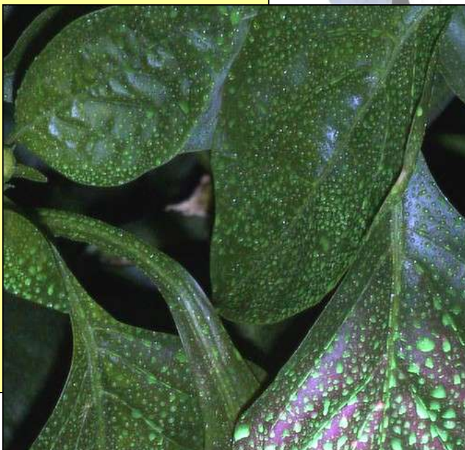
Fluorescent dye used to test spray coverage
